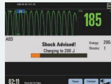
In AED mode, D6 automatically analyzes the rhythm and determines whether a shock is advised. Voice and text prompts guide the user through the process. Voice recording (180 minutes) is also available for case review.
