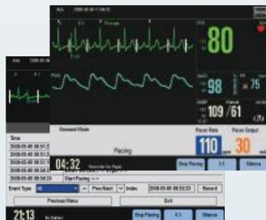
BeneHeart D6 offers demand mode and fixed mode pacing with adjustable rates and output. The 4:1 key enables clinicians to quickly select 1/4 of the pacer rate for observation of the underlying rhythm.
